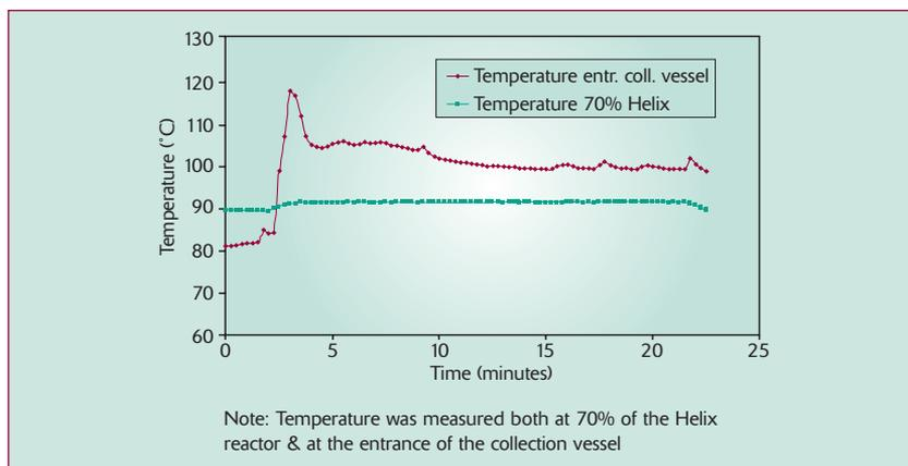
Figure 2 - (above) Results of a typical experiment with the Helix reactor to produce [EMIM][Br]
