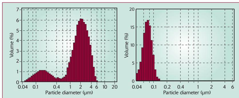
**Figure 3 - Influence of flow on particle size distribution after polymerisation in a straight tube (a) & a Helix reactor (b)**
