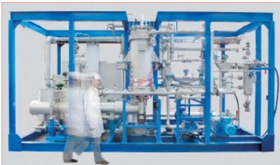
Skid mounted pilot plant with a 55 cm diameter HWC for on-site demonstrations
